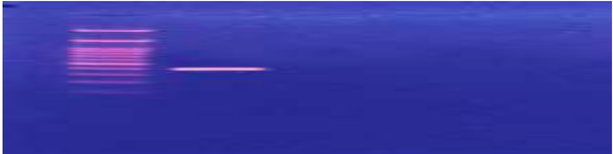
Figure (5) Amplification results of Fluconazole protein-1 for E. nigrum isolates, migrated on 1.5% agarose gel at 70 V for 1.5 hours, and DNA band size (400 bp).
